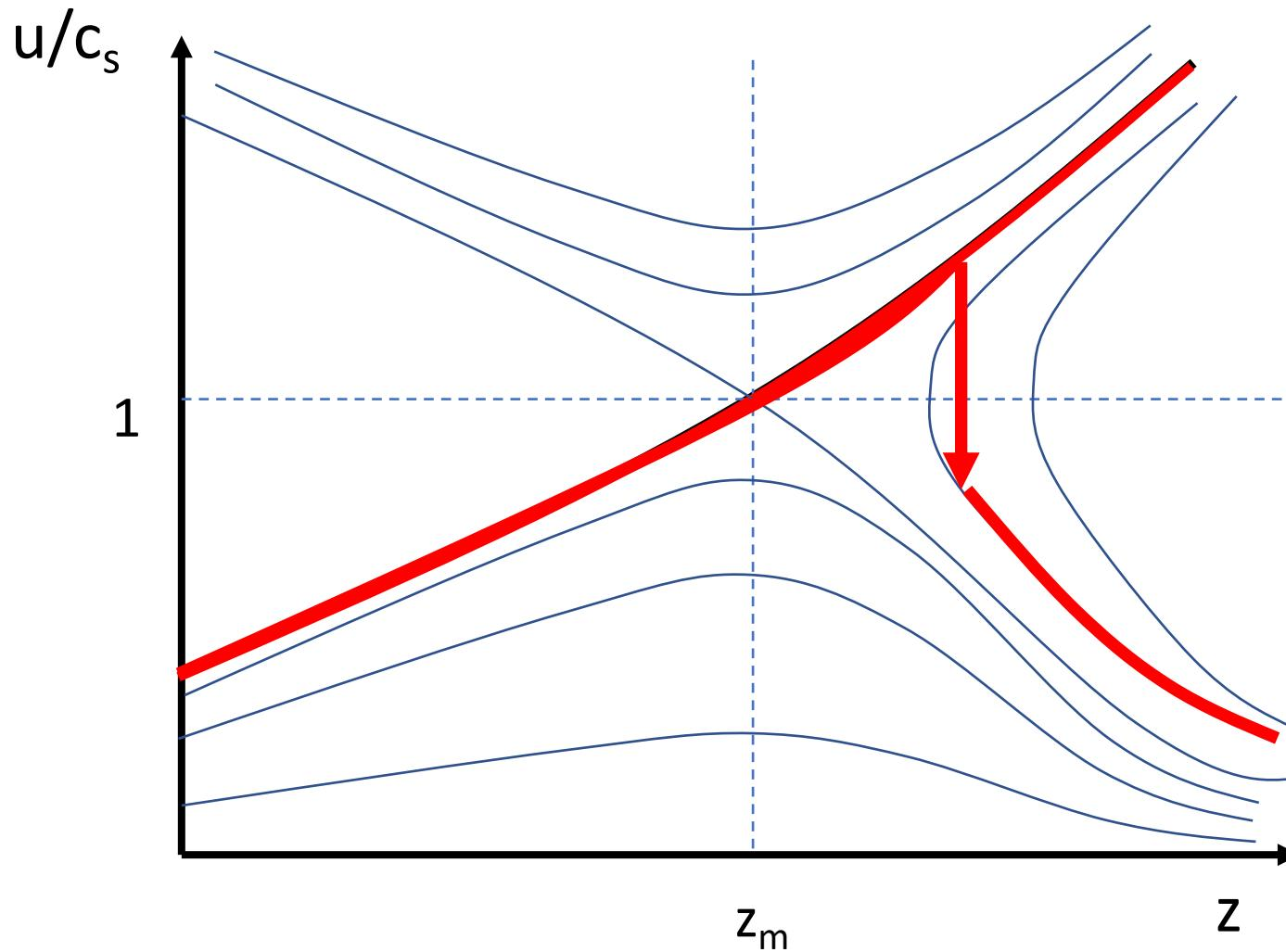
Nozzles can choke due to shock formation in the exhaust
