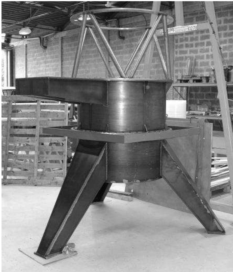
Figure 4. The main structural elements of DAzLE during trial assembly. The overall height of the structure shown is 2.4 metres.
