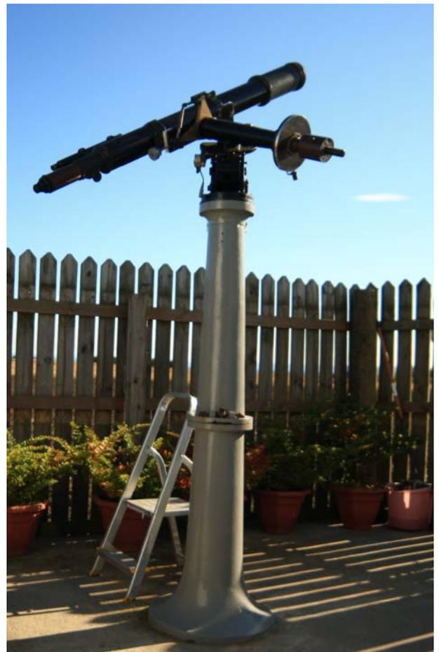
The equatorial mount of Instrument No 27 carrying the George Alcock refractor and mounted on a pier belonging to Denis Buczynski.
