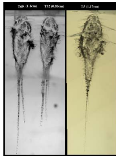
Comet particle tracks in Stardust aerogel
